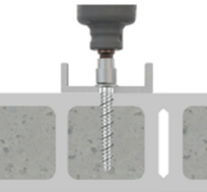
FIGURE 3—MANUFACTURER'S PUBLISHED INSTALLATION INSTRUCTIONS
