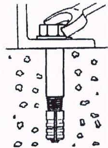
NOTE: Use drill bit conforming to ANSI B212.15-94.
